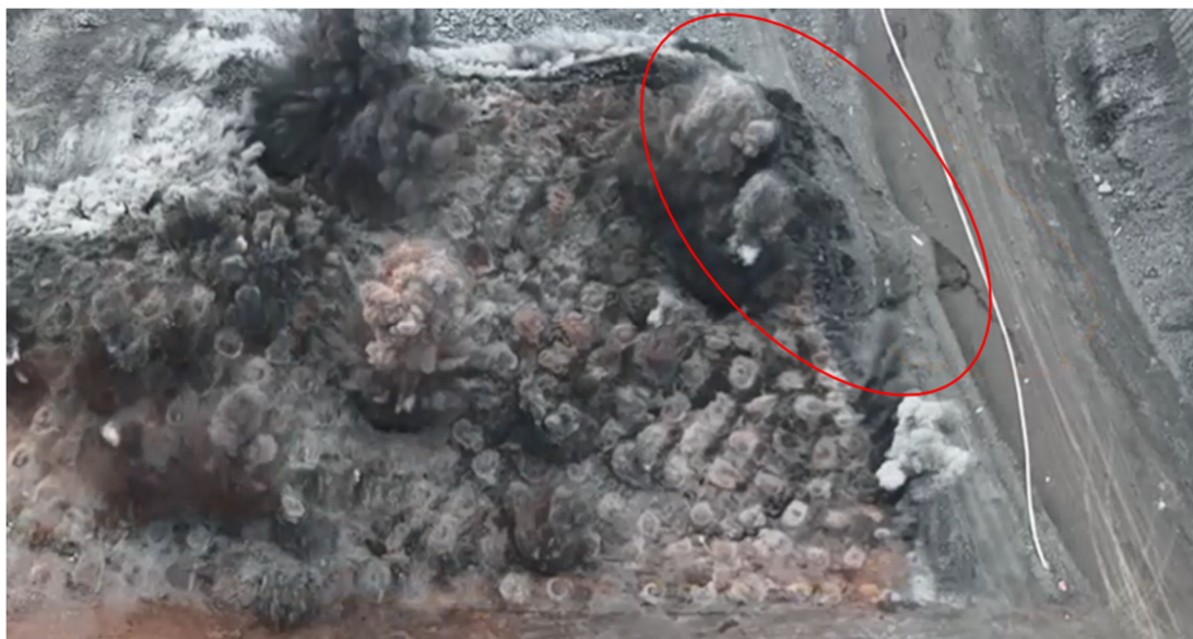
Figure 7 Blast damage from intersecting major structures
