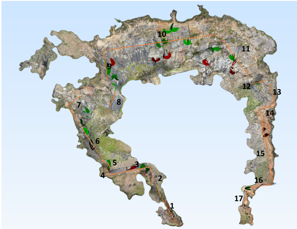
Figure 12 Drone photogrammetry showing wall locations for Probability of Failure analyses
